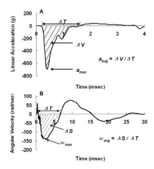
Figure 6-2: Diagrams illustrating data from processing accelerometer velocity and sensors. (A) Methodology for calculating peak and average linear acceleration from linear acceleration time history curve. (B) Methodology for calculating and average angular peak velocity from angular velocity time history curve.
