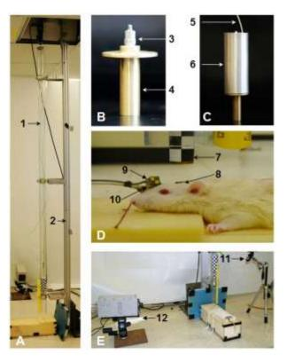
Figure 6-1: Diagrams of the modified impact-acceleration injury model and instrumentation setup. 1 = Plexiglastube; 2 = aluminum pole; 3 =accelerometer (Kistler 8044); 4 = brass impact end; 5 = accelerometer cable; 6 =aluminum cylinder part of impact housing accelerometer; 7 = brass impactor end with tracking label; 8 =helmet; 9 = angular rate sensor (DTS AR12k); 10 = accelerometer (Endevco 7269); 11 = IR laser pointer; 12 = high speed camera (MotionXtra HG-100K HG-100k)
