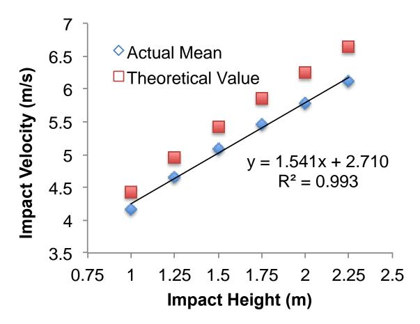
Figure 5-2: Impact velocity as a function of drop height determined for the new impact acceleration device
