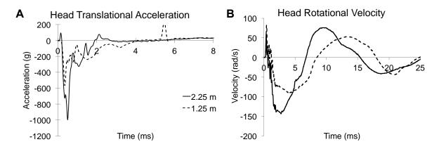
Figure 5-5: Typical time-history traces of (A) translational acceleration and (B) rotational velocity measured on the rat head in the sagittal plane in 1.25 and 2.25 m head impacts, respectively.
